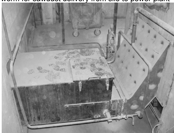
Slika 11. Tračni transporter za dobavu piljevine iz silosa u peć – skuplje ali bolje rješenje Figure 11 Belt conveyor for sawdust delivery from silo to power plant – more expensive but better solution
